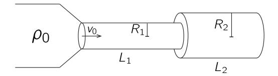
Consider particles that are embedded in an incompressible solvent, and that flow with the solvent through two connected pipes with different radii  $R_1$  and  $R_2$ , as shown in the figure. To the left, the pipes are connected to a solvent and particle reservoir. The density of particles in the reservoir is given by  $\rho_0$ . The mean flow velocity at the entrance is  $v_0$ .
